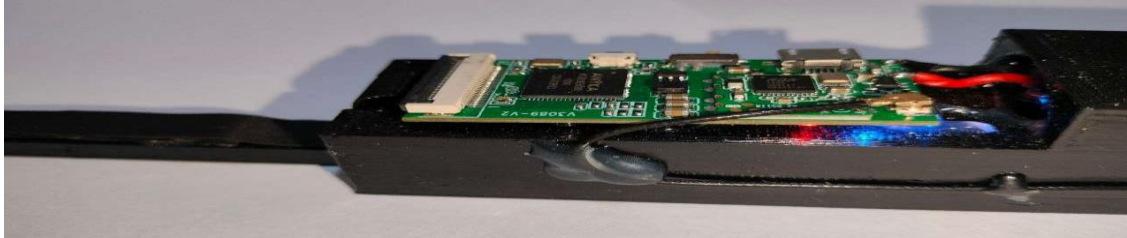
Figure (3-5): Electrical circuit and antenna wire assembly.
